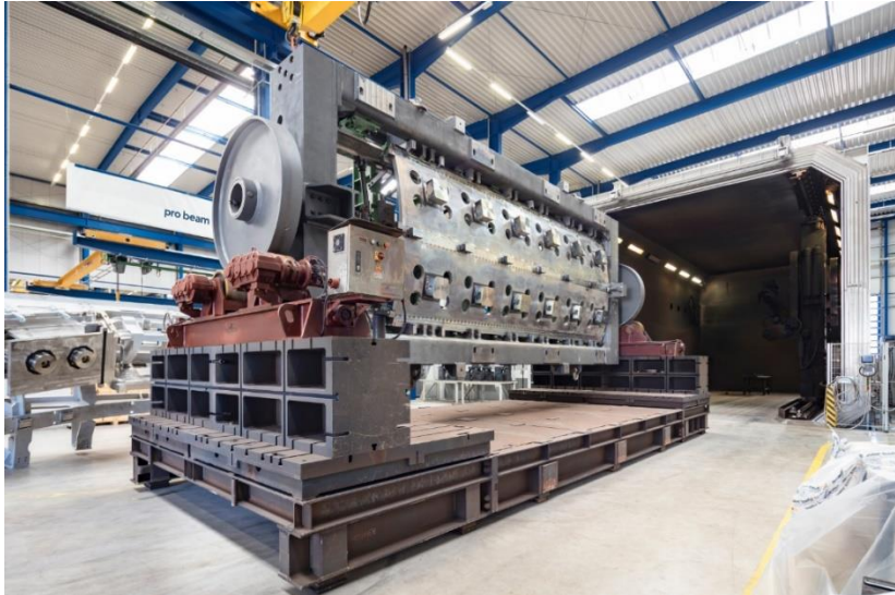
Figure 5: Vacuum Vessel component in a rotating welding device at pro-beam in Burg. Source: pro-beam
