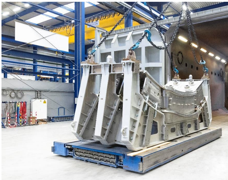
Figure 4: Vacuum Vessel component in a welding device at pro-beam in Burg. Source: pro-beam
